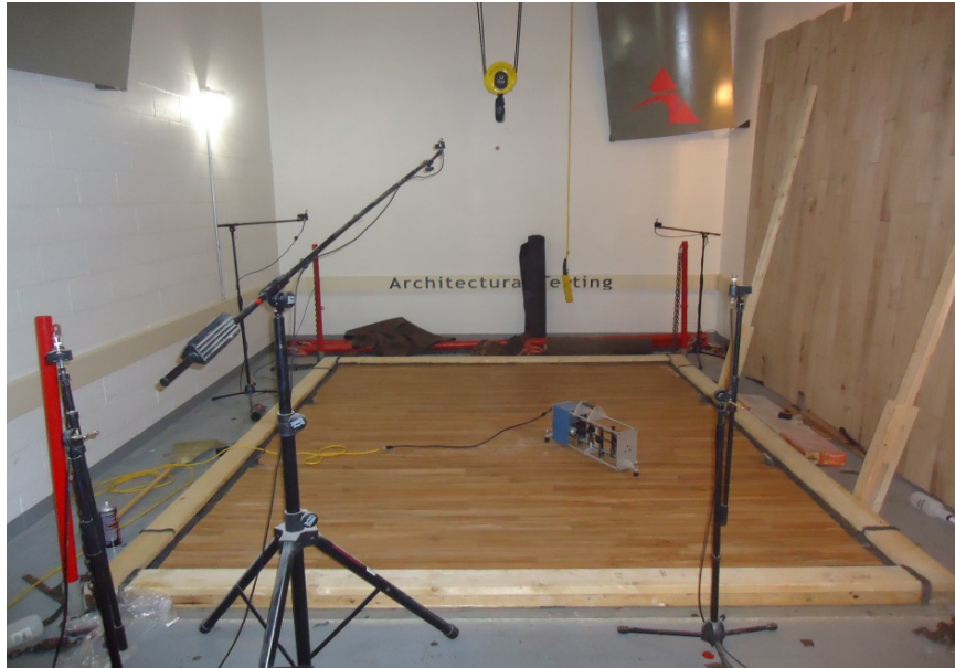
Source Room View of Test Specimen Installation
