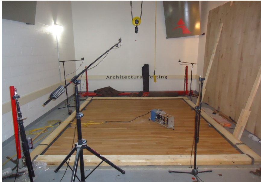
Source Room View of Test Specimen Installation
