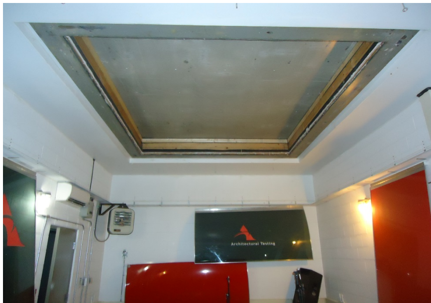
Receive Room View of Test Specimen Installation
