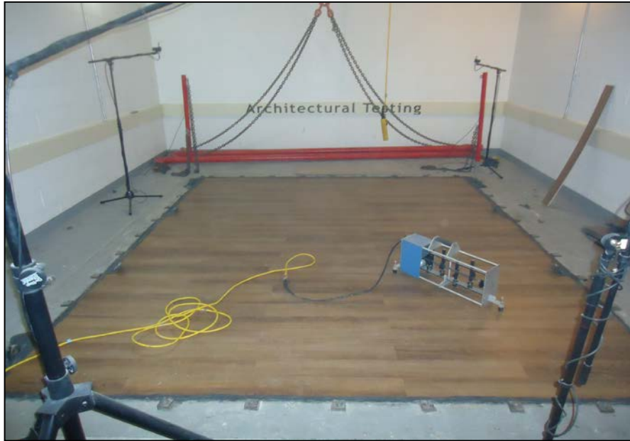
Source Room View of Test Specimen Installation
