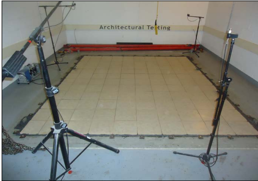
Source Room View of Test Specimen Installation
