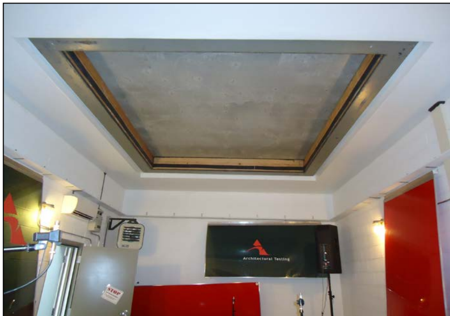
Receive Room View of Test Specimen Installation
