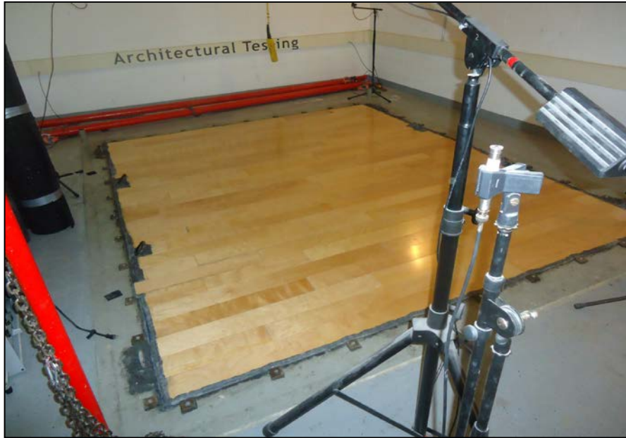
Source Room View of Test Specimen Installation
