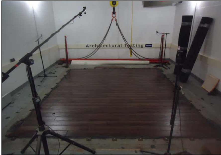
Source Room View of Test Specimen Installation
